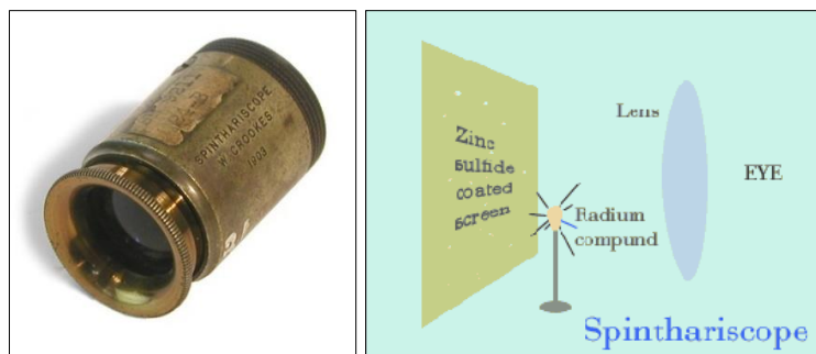
Figure 2-8 Spintharoscope, used by Rutherford and his students.
