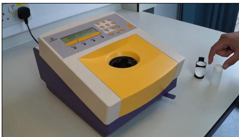
Figure 5-3 Hidex Triathlon LSC. The vial and its cover are also shown
