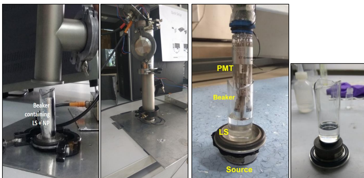
Figure 4-4 View of glass beaker containing the liquid scintillator.
