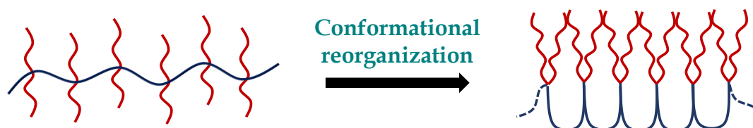
Scheme 2. Schematic representation of the amphiphilic criss-cross polymer and its immiscibility driven folding behaviour.
